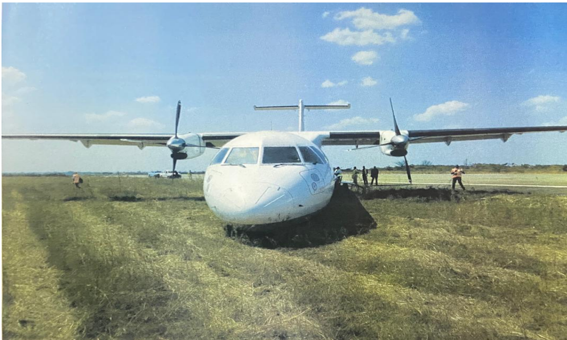
Figure 8: Aircraft with collapsed nose gear
