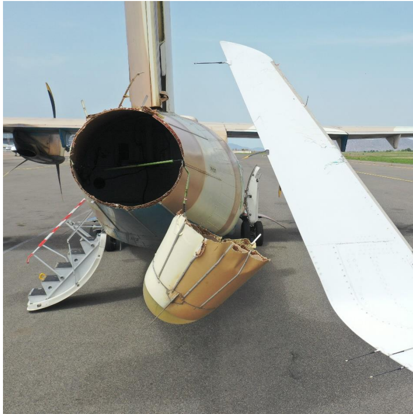
Figure 2: Sheared off section of the Tail cone of the parked ATR 42 (NAF930)
