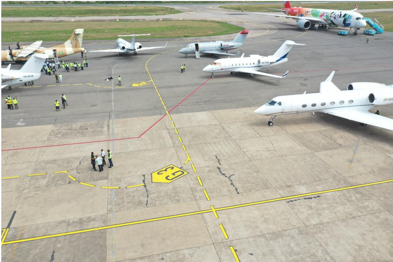
Figure 4: NAF ATR 42 parked at unmarked spot with its Tail Section protruding into the Apron Taxi Lane. Other aircraft parked at unmarked spots on the GAT Apron right side of 5N-BXK
