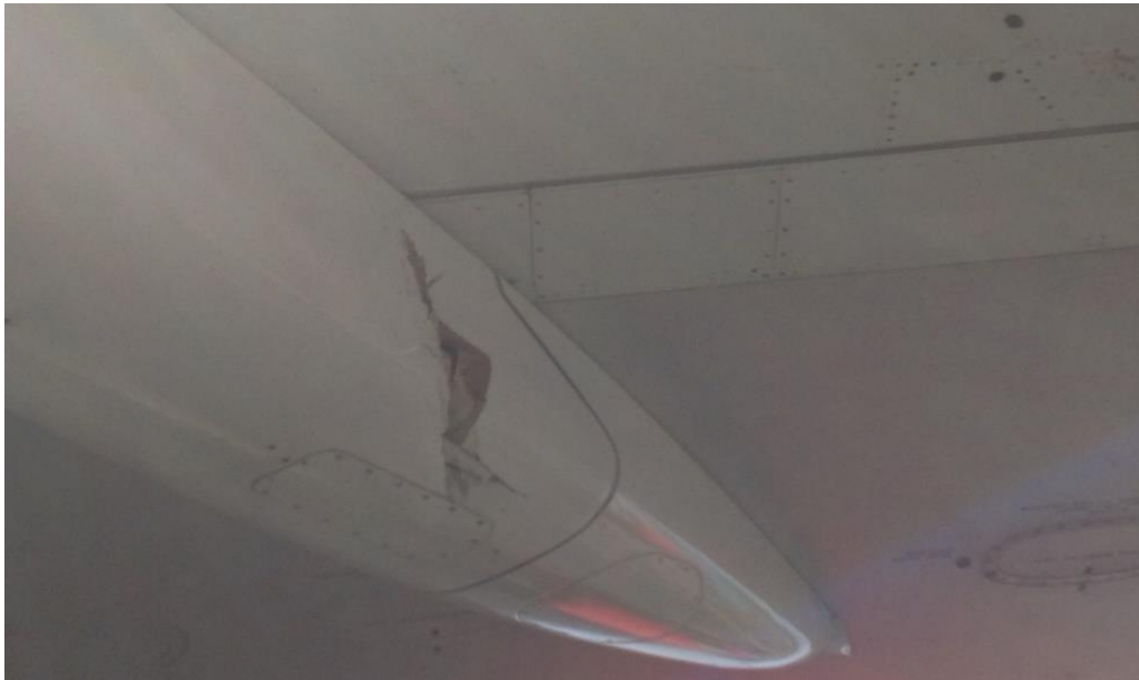
Figure 14: Torn flap fairing on the left wing
