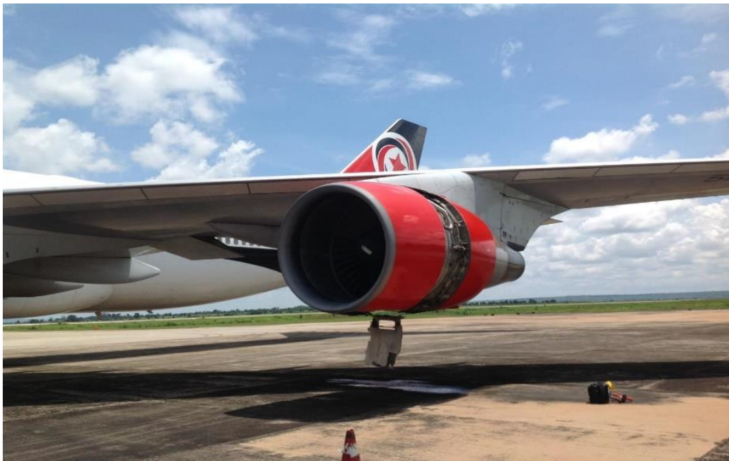
Figure 11: Damaged cowling of engine number one
