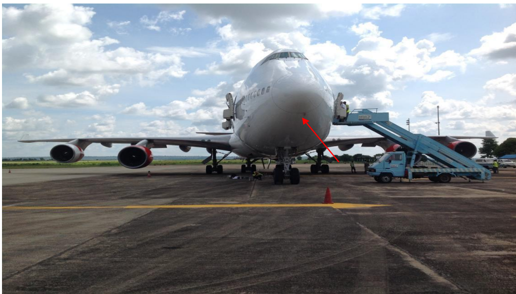
Figure 15: Evidence of bird strike on the lower radome
