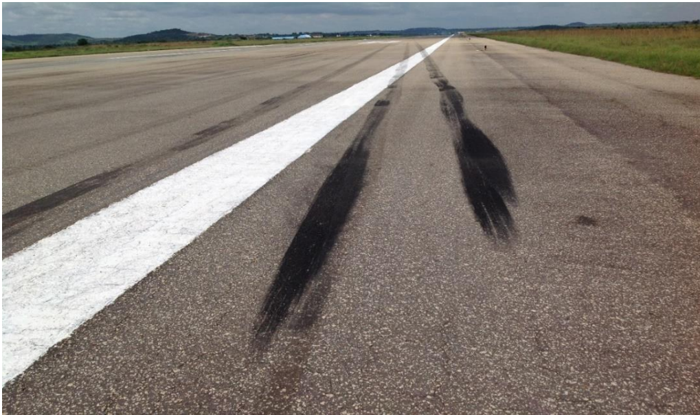
Figure 12: Tyre marks indicating the touchdown point
