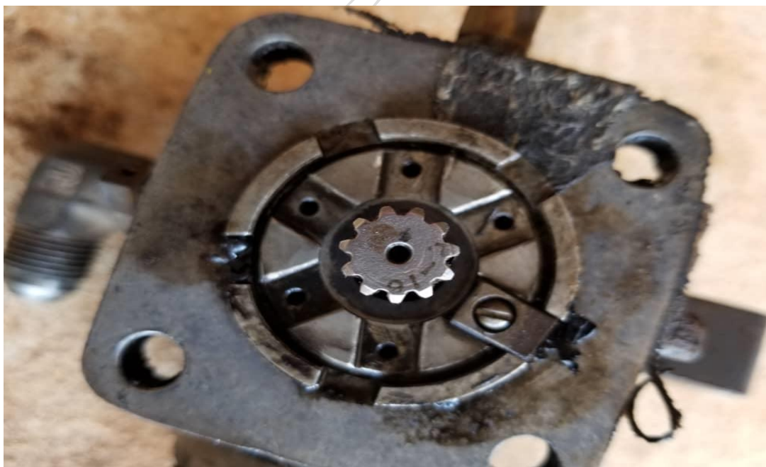
Figure 8: Fuel pump showing the spline and drive shaft
