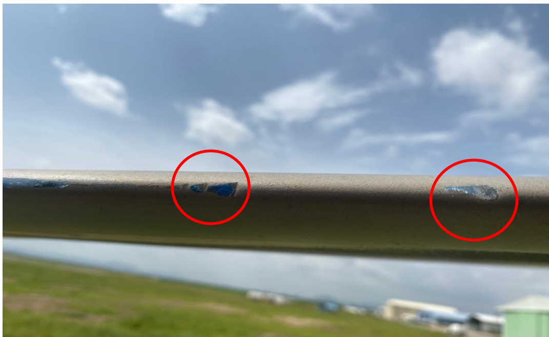
Figure 2: Strike marks on the Helicopter Main rotor blade
