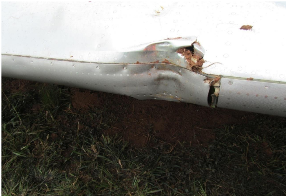
Figure 7: Right-wing leading edge damage
