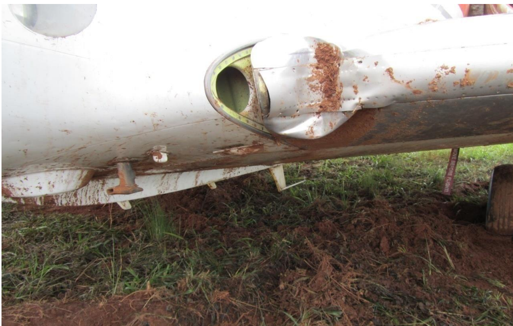
Figure 8: Damage to the right-wing leading edge at the wing root
