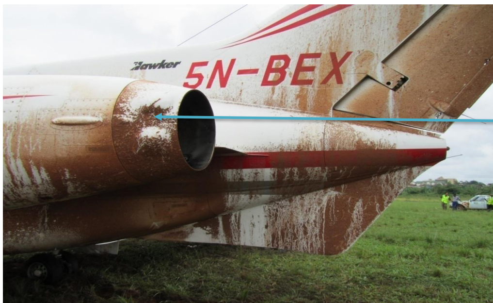
Figure 9: Dent of the No. 1 engine exhaust with mud splatter on the empennage of the aircraft
