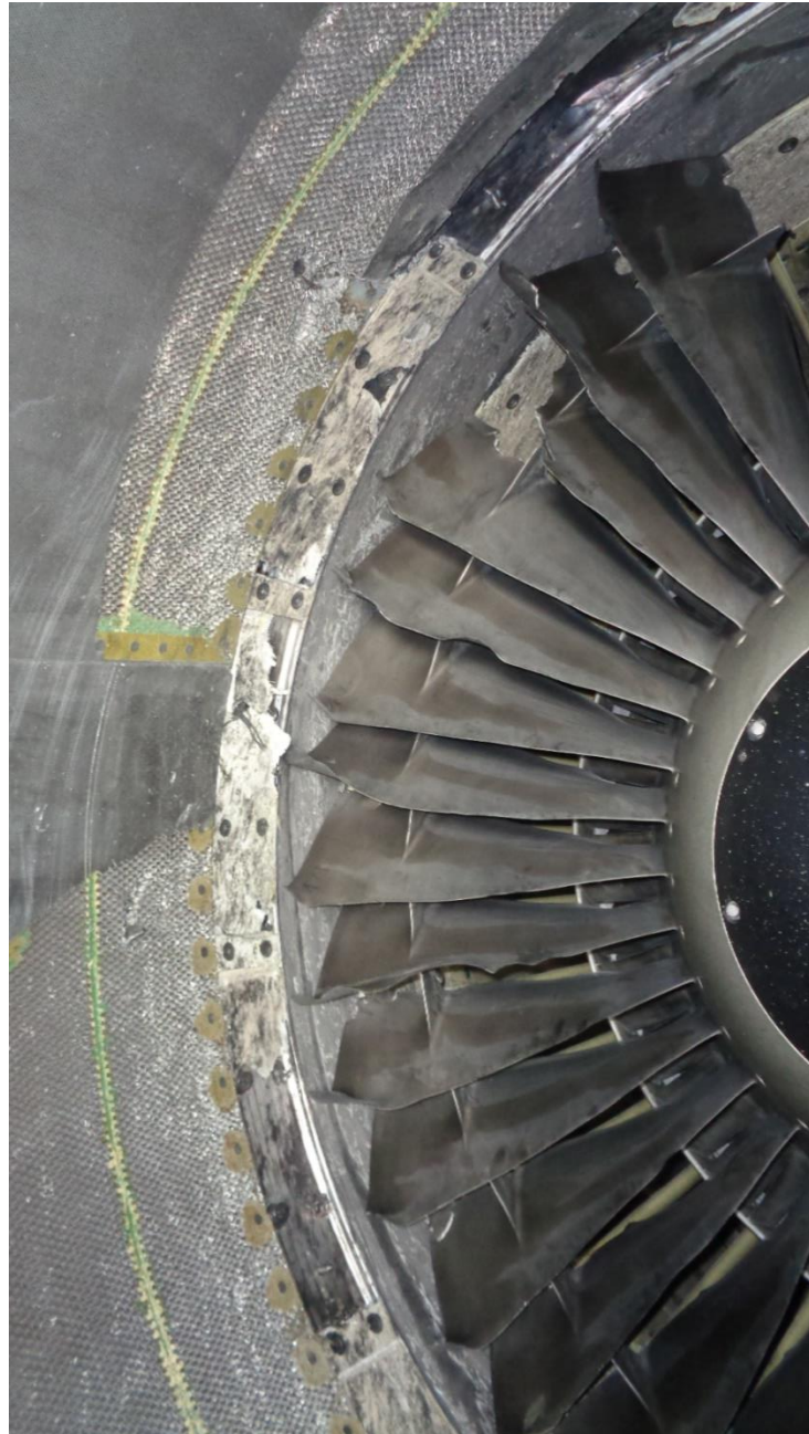
Figure 2: Damaged fan blades of number 1 engine caused by ingestion of debris from the burst tyre
