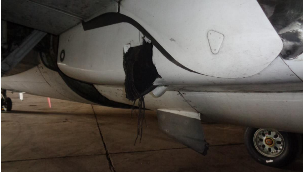
Figure 5: A damaged section of the fuselage due tire debris
