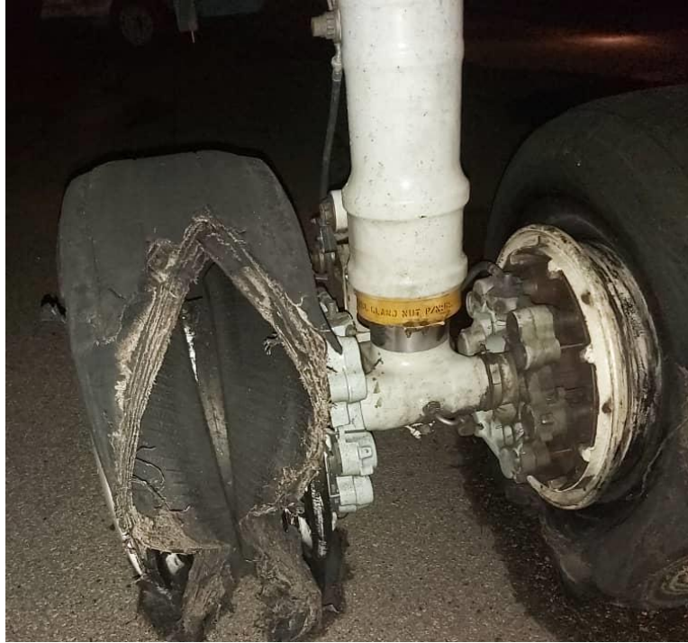
Figure 3: Damaged number 1 & 2 main wheel tyres
