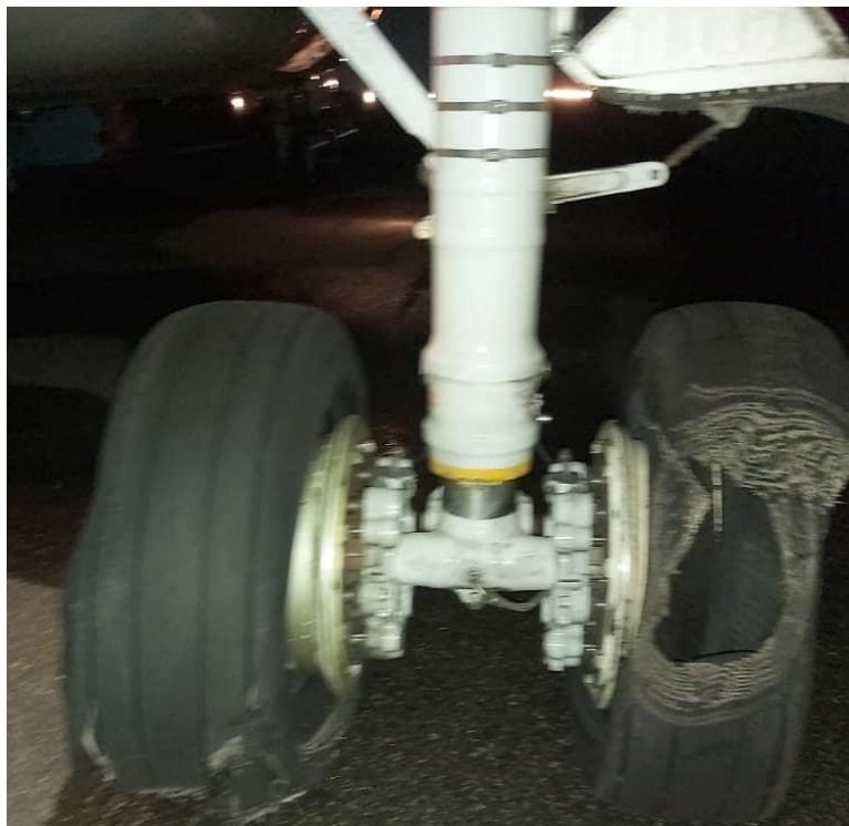
Figure 4: Rear view of damaged number 3 & 4 main wheel tyres
