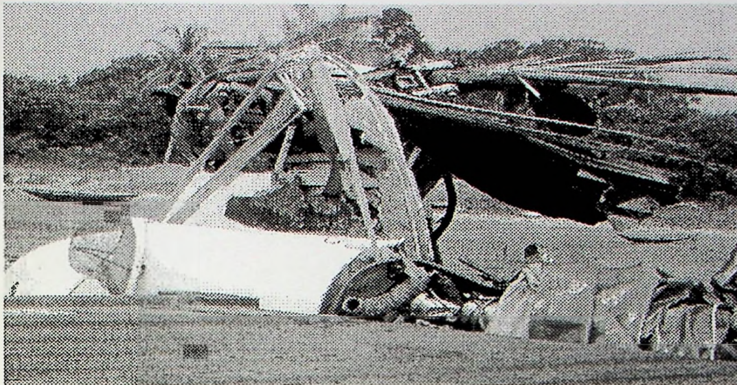
The devastating destruction of the Main Rotor Blades portrays the closeness of the helicopter to the container on the barge.
