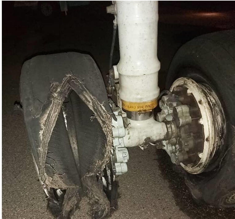
Figure 3: Damaged number 1 & 2 main wheel tyres
