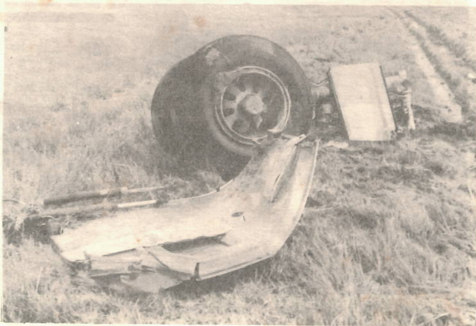
The severed right landing gear after running into the trench.
