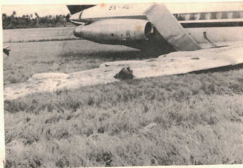
The right wing in contact with ground and showing the imbedded bird dispersal gun's gas tank.
