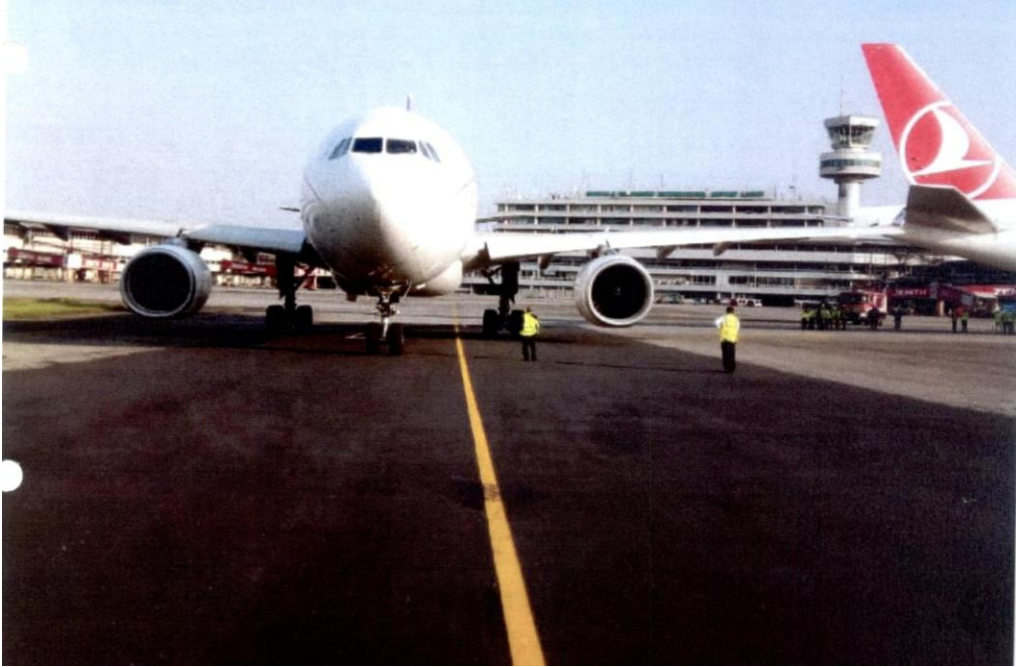
Figure 5: Photo of deviation of MEAs airlines aircraft from the Taxi line
