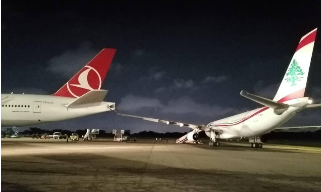
Figure 3: Photo of MEA aircraft winglet clipping the APU exhaust of the Turkish aircraft
