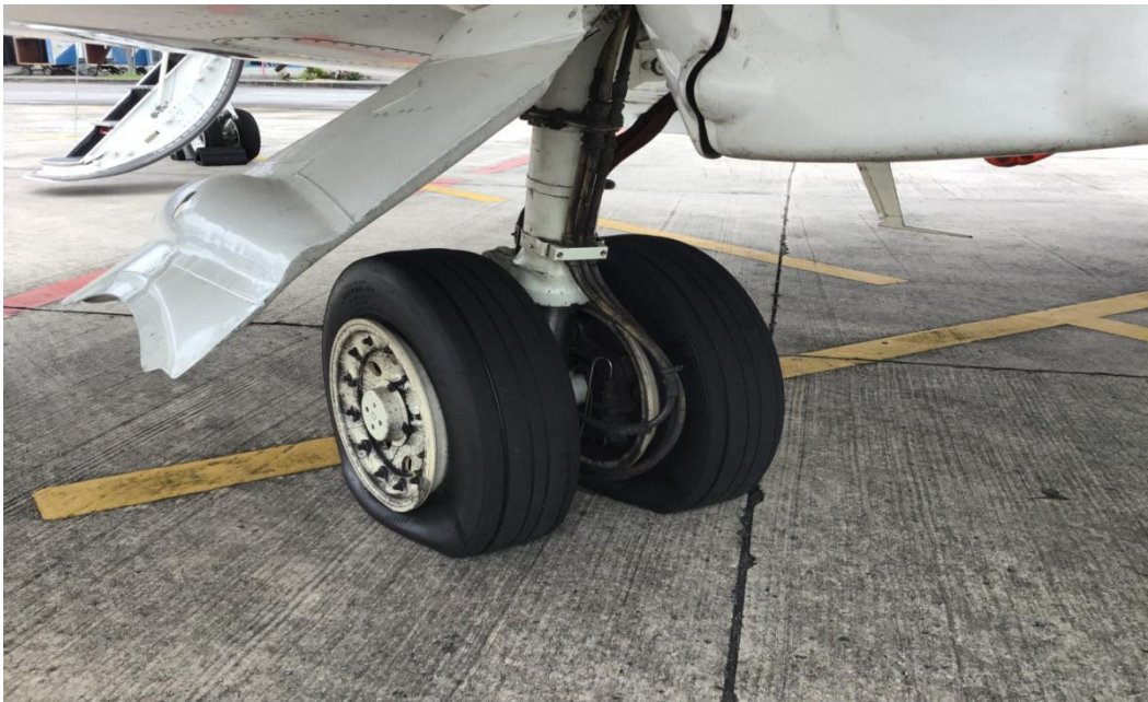
Figure 2: The left main wheel tires (No.1 and No.2) deflated
