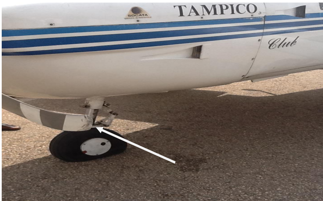
Figure 2: Bent propeller blade tip
