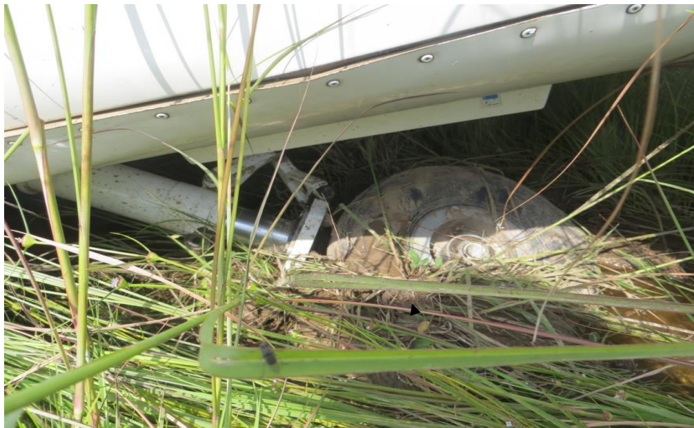
Figure 3: Collapsed Nose Landing Gear
