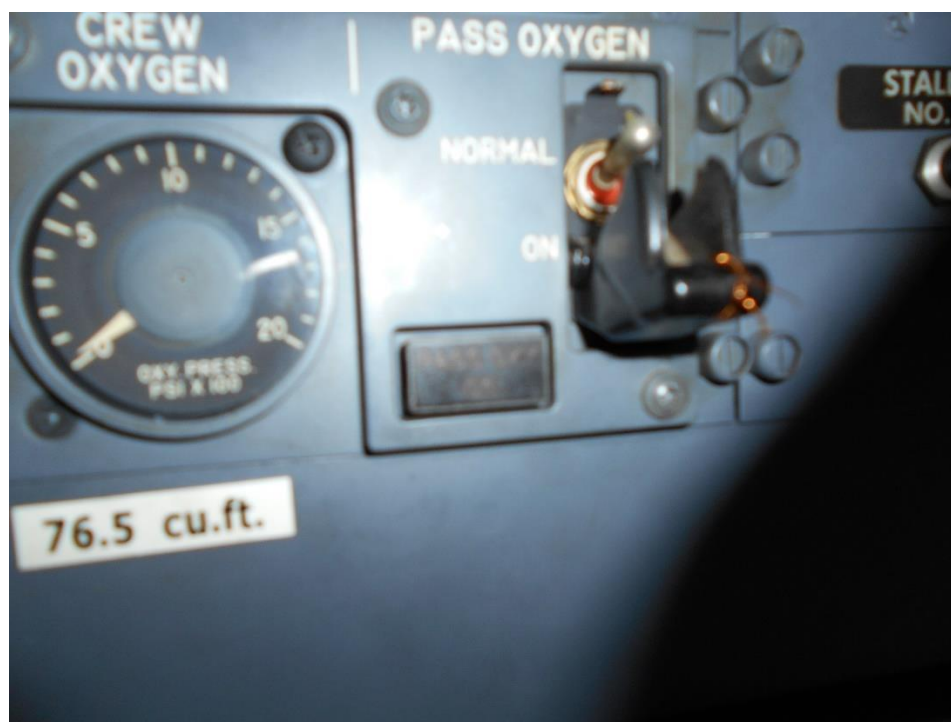
Figure 2: Photo of passenger oxygen switch in the NORMAL position, with broken wirelock
