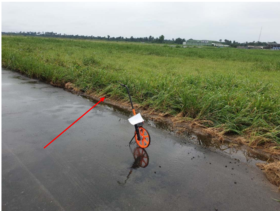
Figure 3: Picture showing tracks of the left main wheel at the touchdown point
