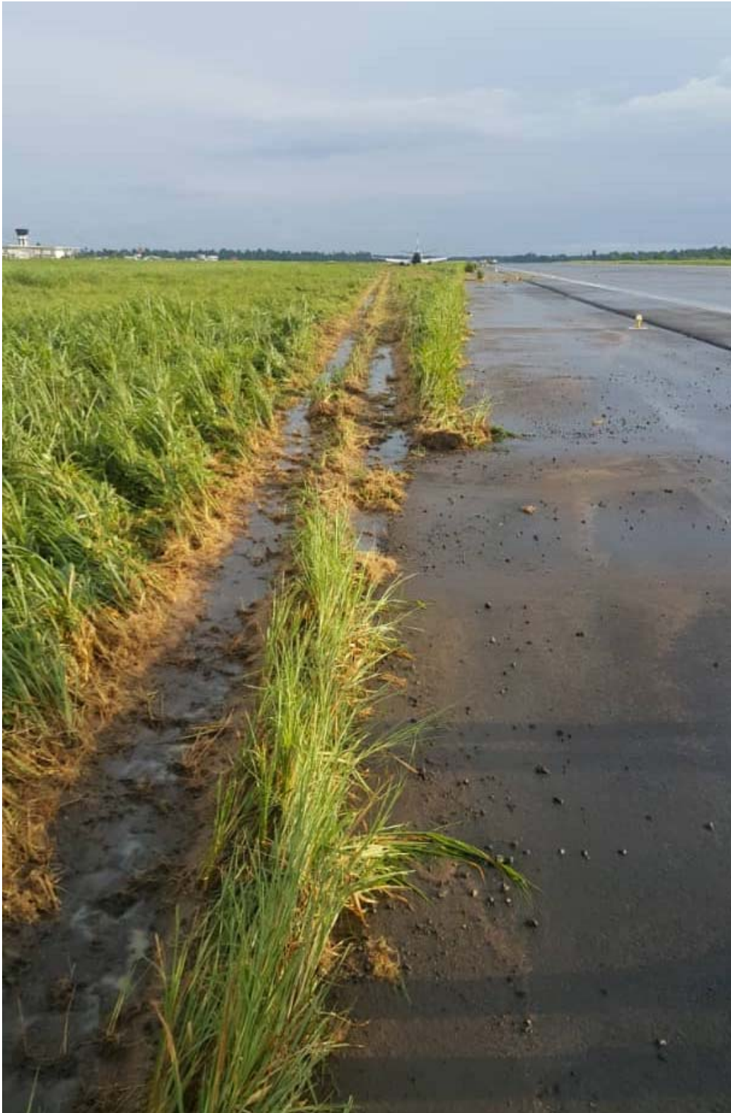
Figure 4: Picture showing the tracks of the main wheels leading into the grass verge
