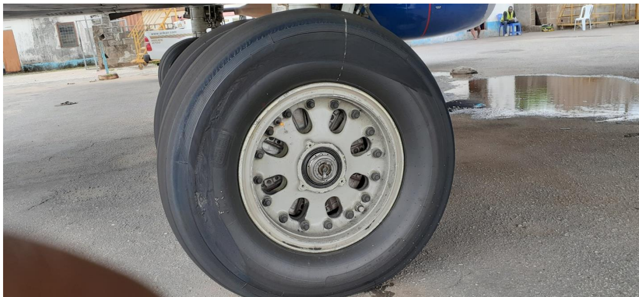
Figure 2: Picture showing Scuff marks on the No. 4 main wheel tyre
