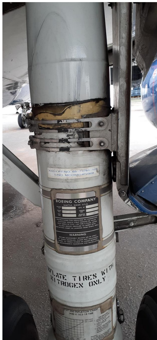
Figure 3: Pictures showing evidence of collapsed Oleo Strut
