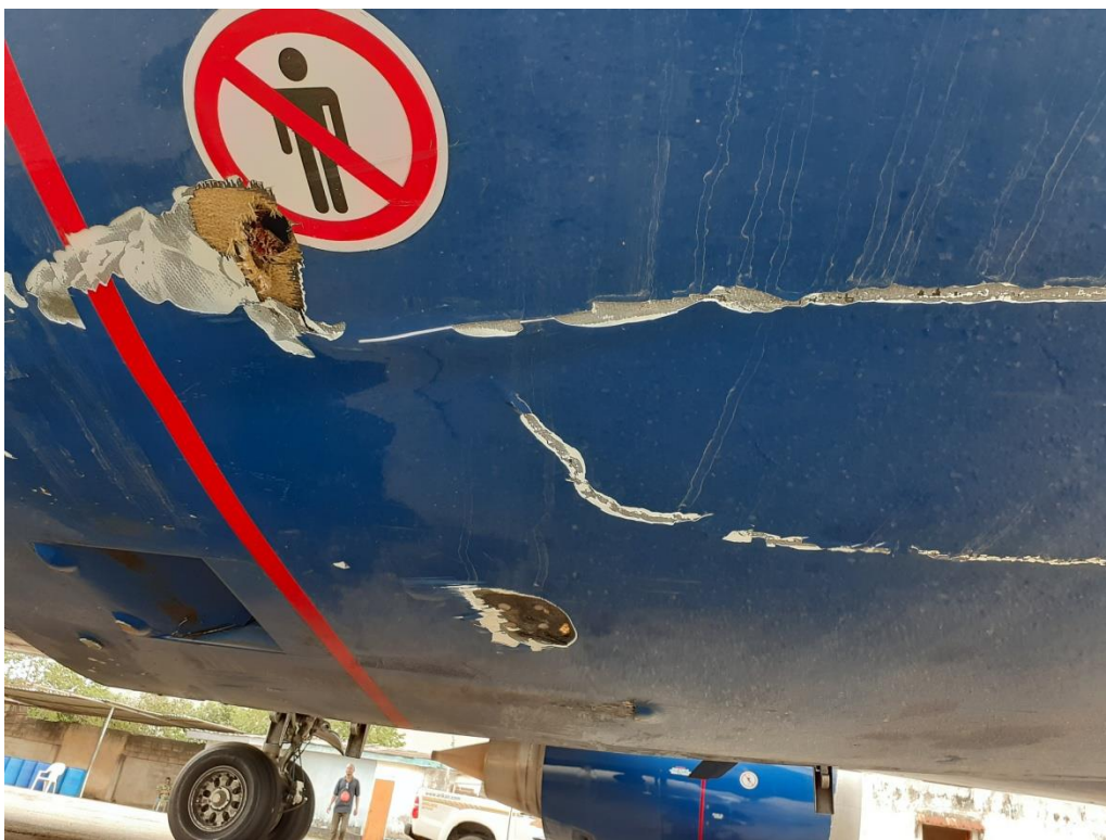
Figure 1: Picture showing Scrapes and dents on the No. 2 engine cowling
