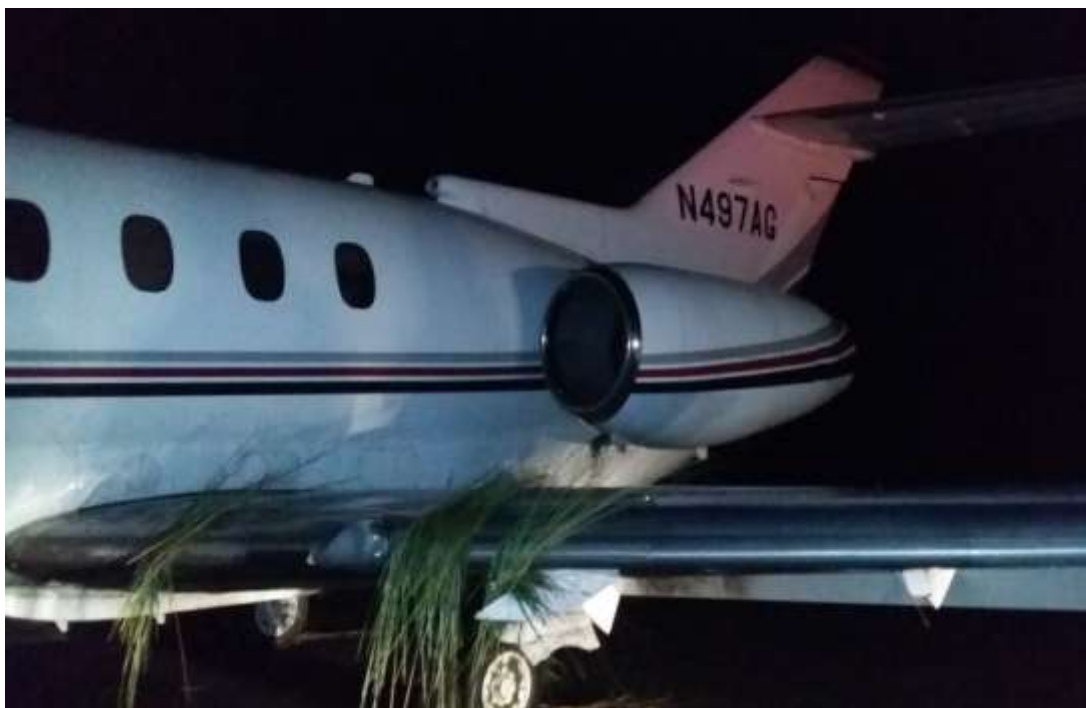
Figure 1: Photograph showing grass ingestion at the generator cooling inlet
