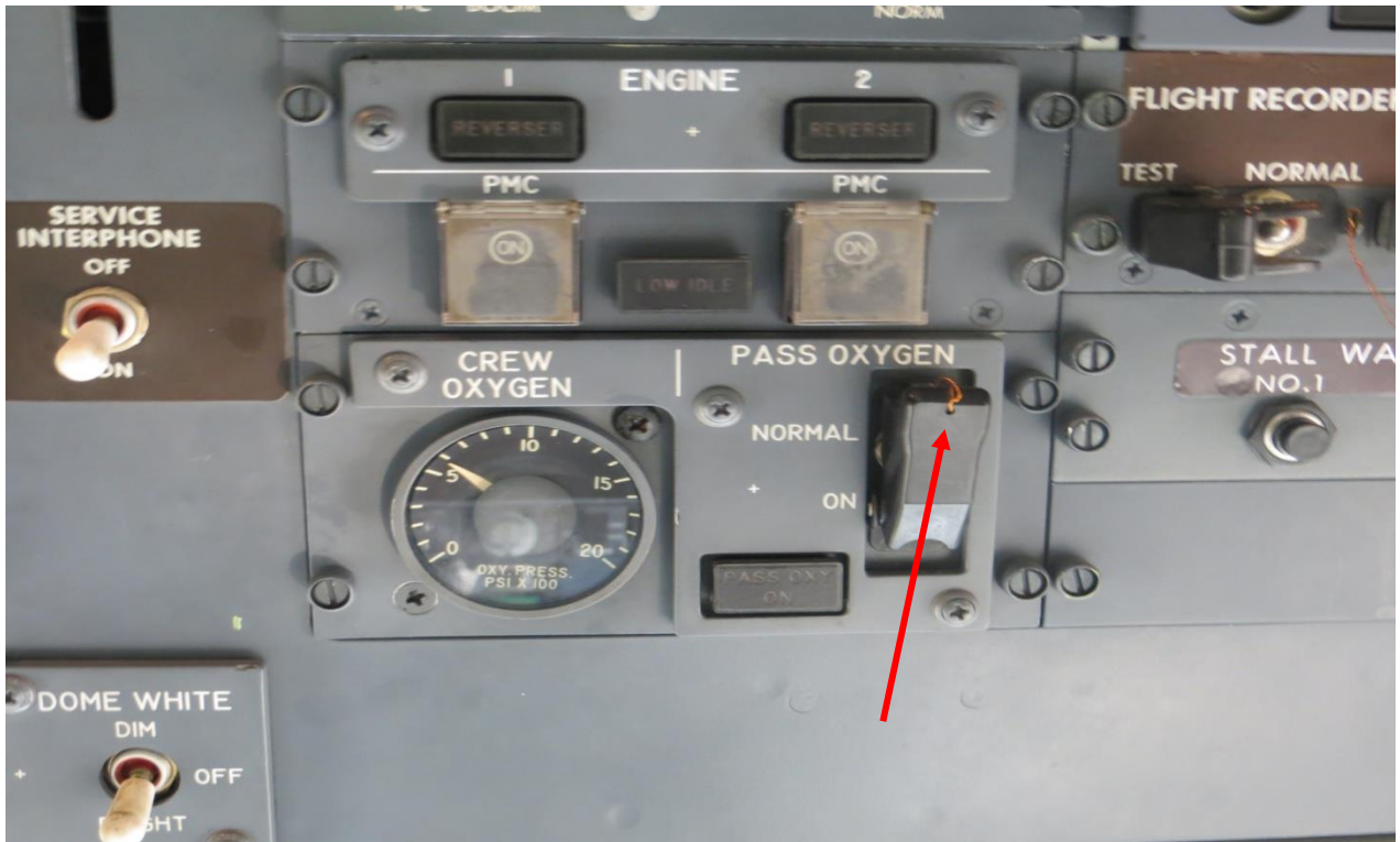
Figure 4: Photo showing the Passenger Oxygen switch wire locked in 'Normal' position as indicated by the Red arrow.
