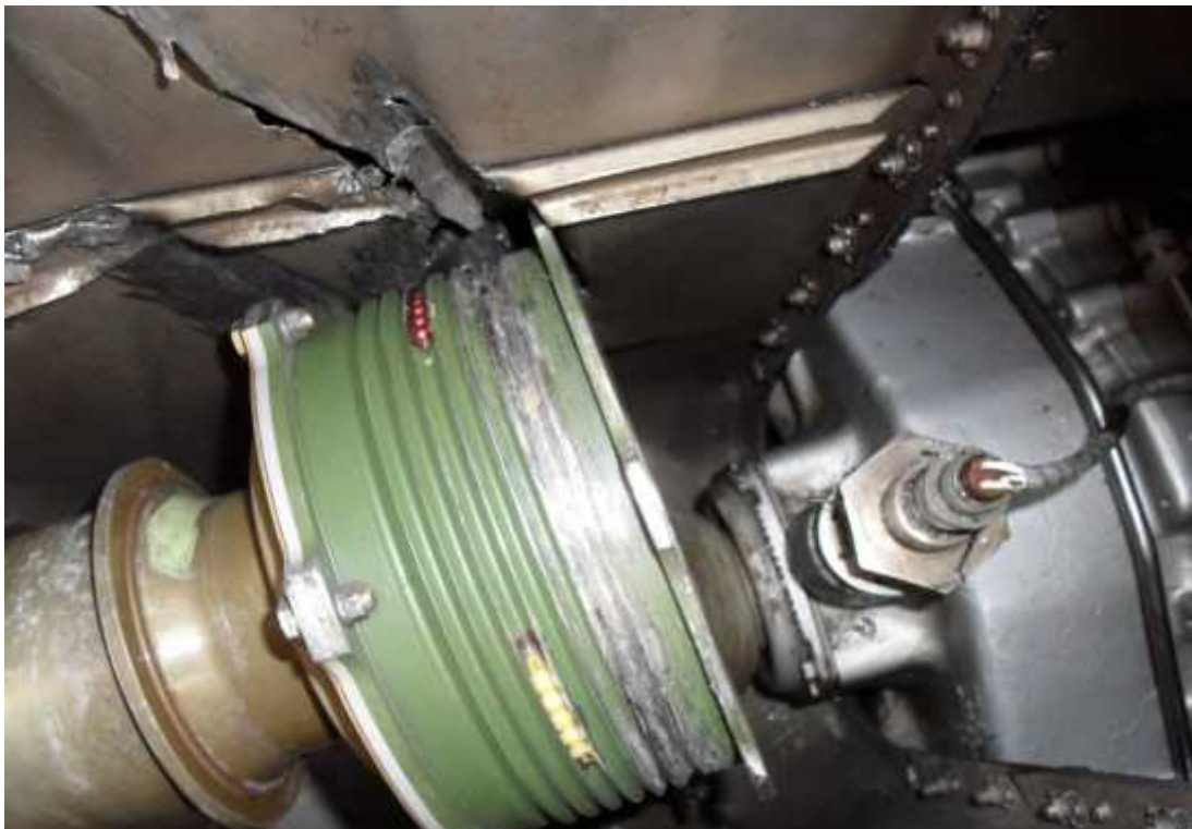
Fig 1.12c: Picture showing the damaged part of a coupling joint of the drive shaft
