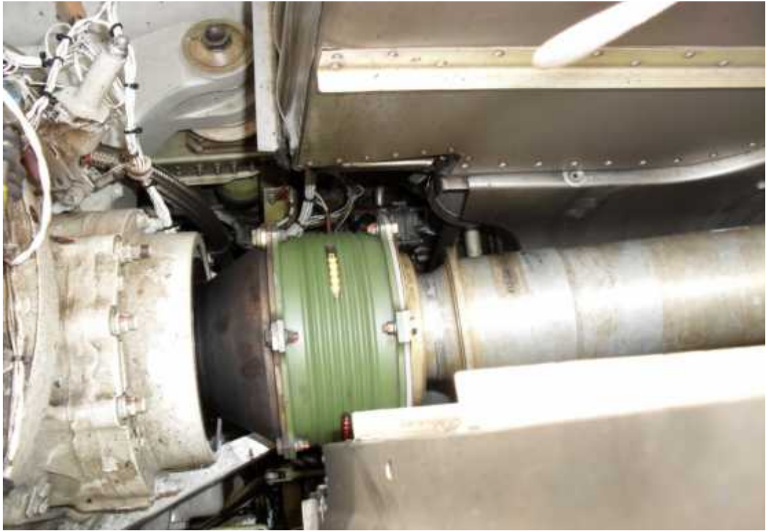
Fig. 1.12f showing bolts intact at the transmission end.
