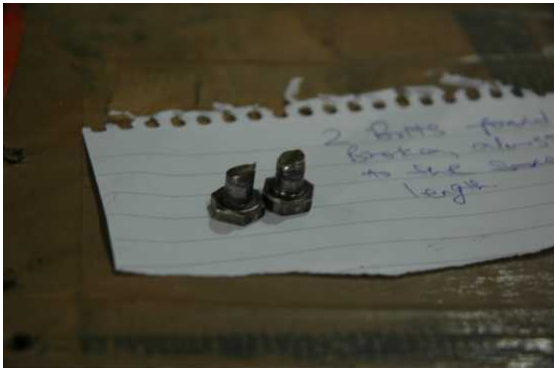
Fig1.12e showing two bolts found on the C-box end inside the aircraft.
