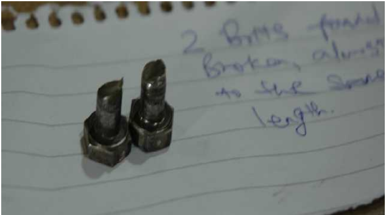
Fig 2.1a showing two bolts found on the C-box end inside
