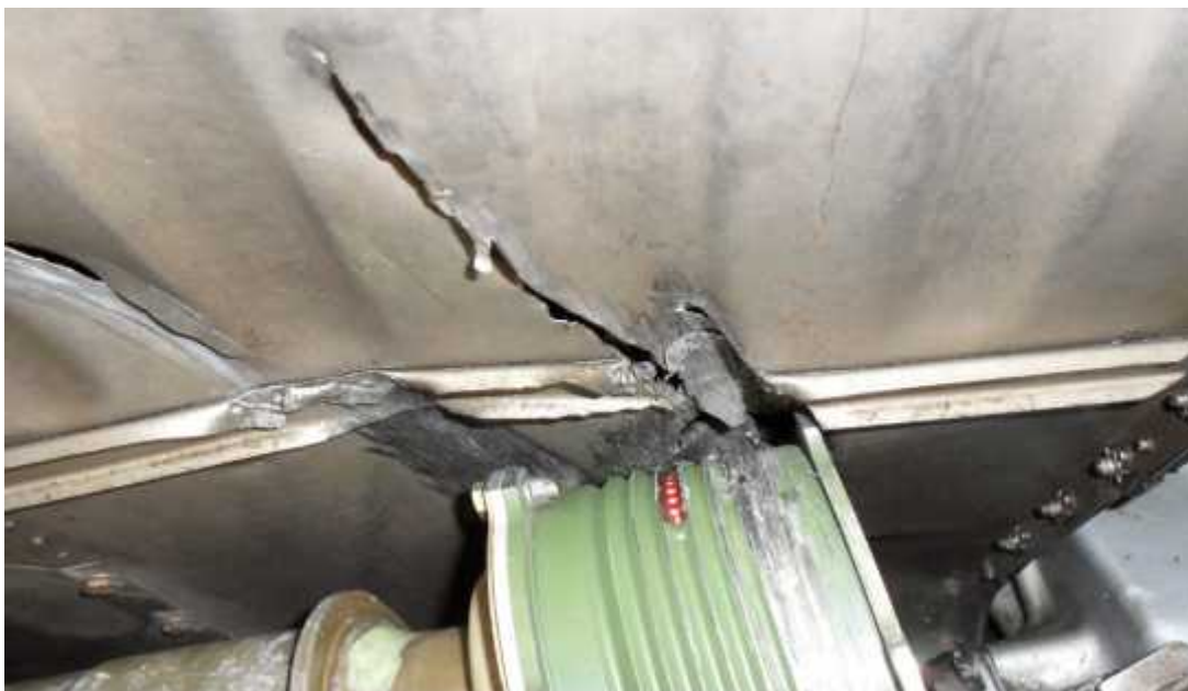
Fig 1.3 showing damage to tunnel area housing the Main Drive Shaft (MDS)
