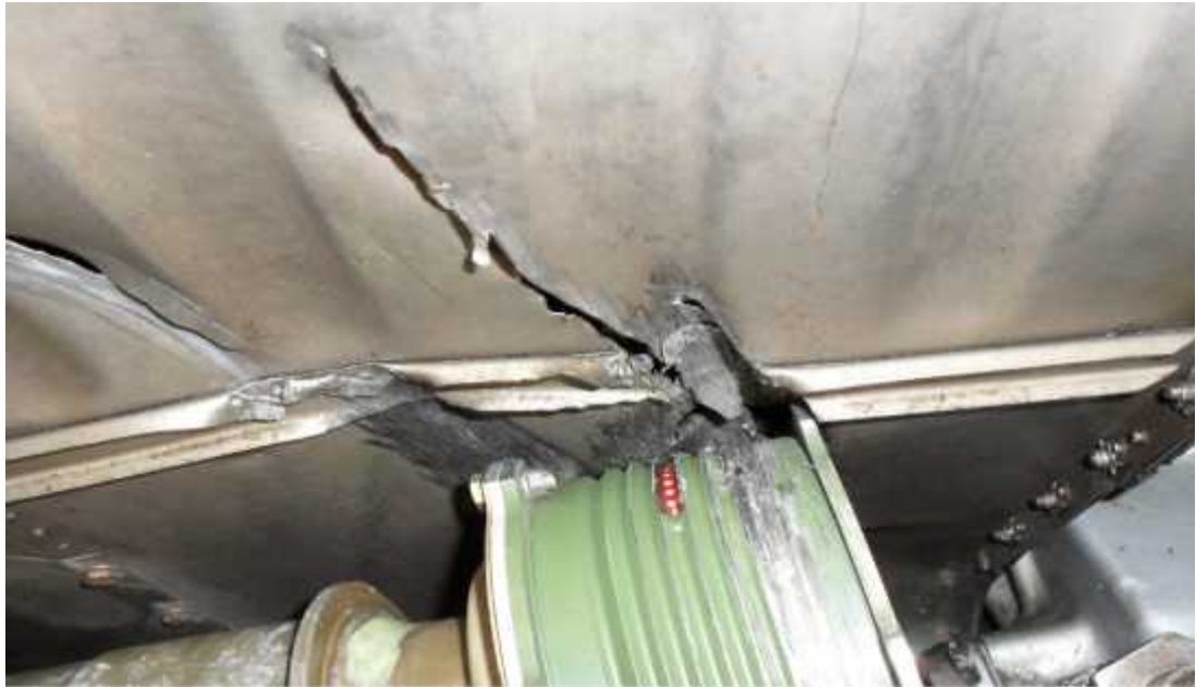
Fig 1.12d showing damage to tunnel area housing the Main Drive Shaft (MDS)
