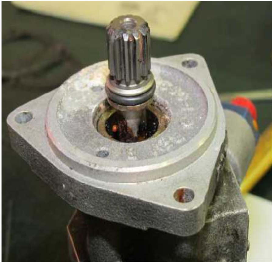
Fig.1.16b: Picture showing Fuel Pump Main Drive Shaft prior to removal from Fuel Pump.
