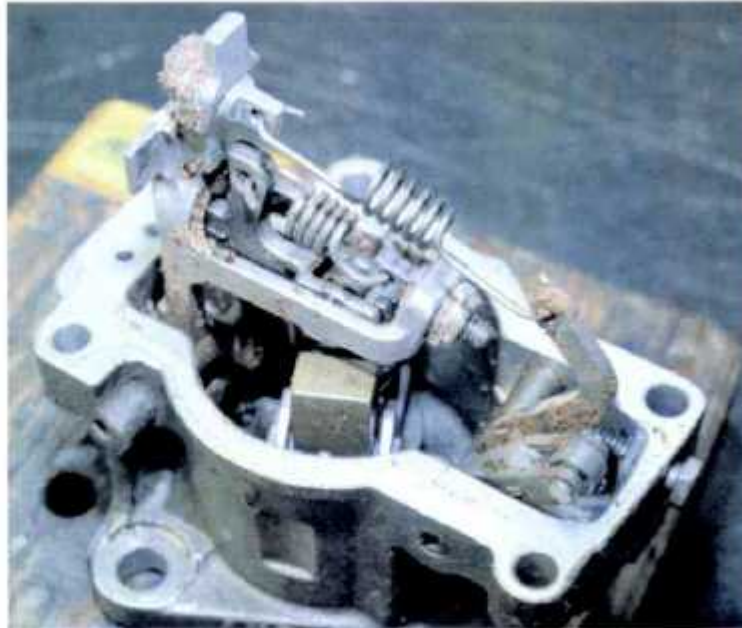
Photo 8 Fuel Control Unit interior
