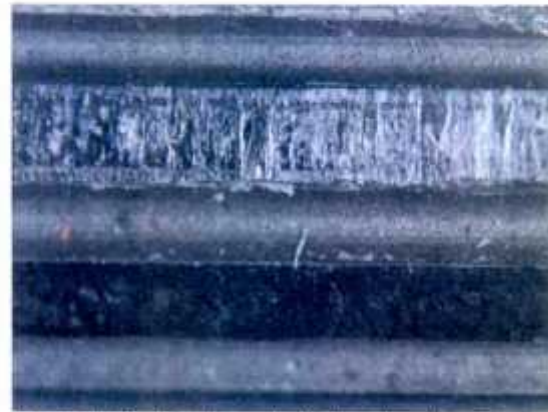
Figure AI-40: Main drive shaft inboard end – worn splines, 20X
