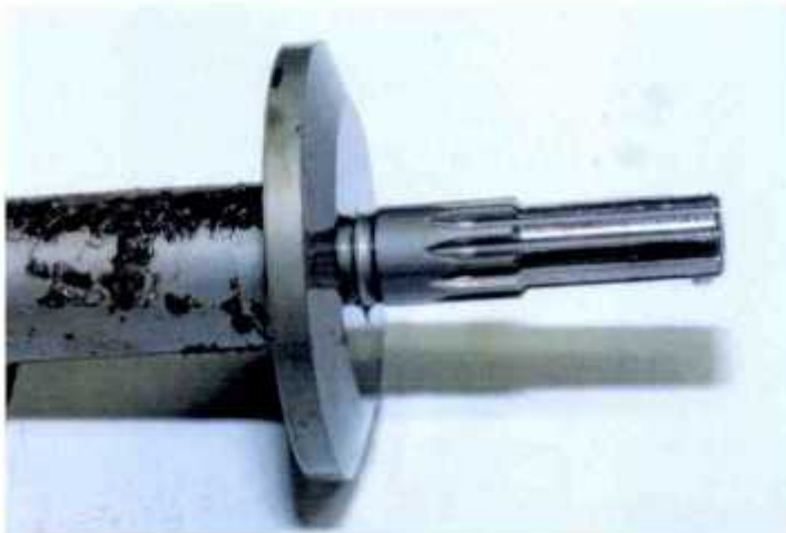
Photo 12 Fuel Pump Main Drive Shaft upon removal
