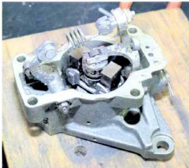
Photo 9 Power Turbine Governor interior
