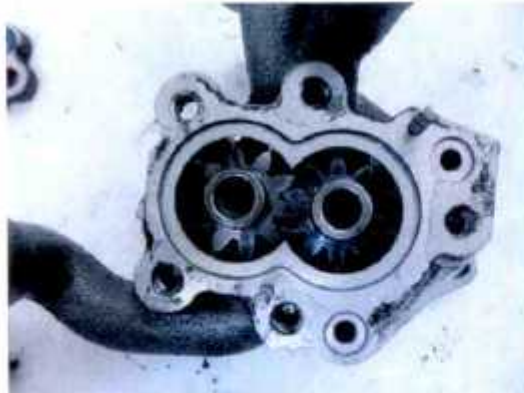
Figure AI-33: Pump gears with fixed bearings removed
