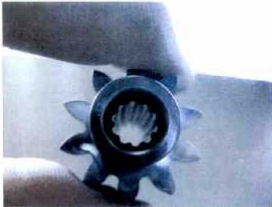
Figure AI-37: Pump driver gear spline (main drive shaft end)
