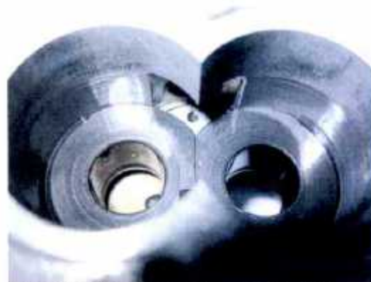
Figure AI-35: Pump floating bearings (installed)
