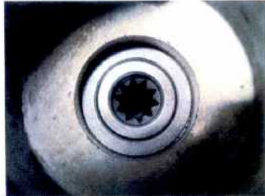
Figure AI-32: Pump driver gear and fixed bearing (installed)
