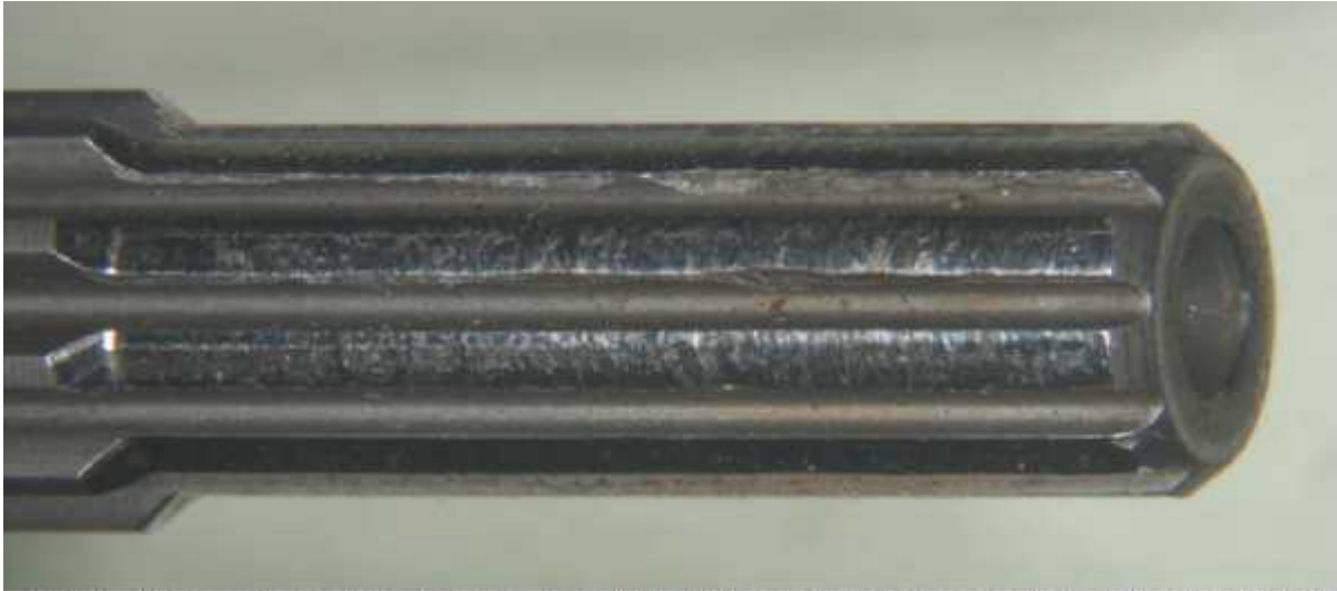
Fig.1.16e: picture showing the Magnified View of Fuel Pump Main Drive Shaft Splines Wear
