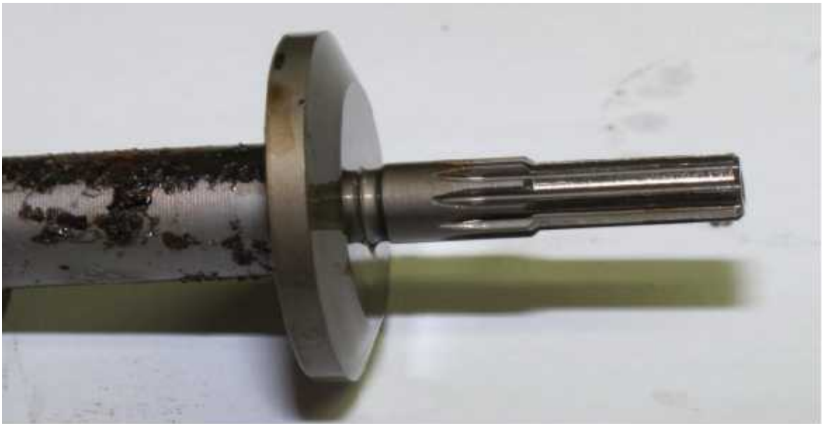
Fig.1.16d: Picture Showing Fuel Pump Main Drive Shaft after removal
