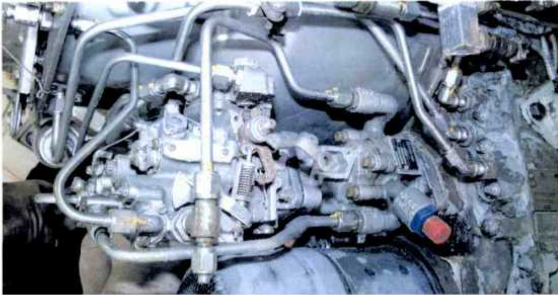
Photo 4 Fuel Control Unit and Fuel Pump prior to removal
