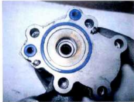
Figure AI-26: Main pump / control drive housing interface
