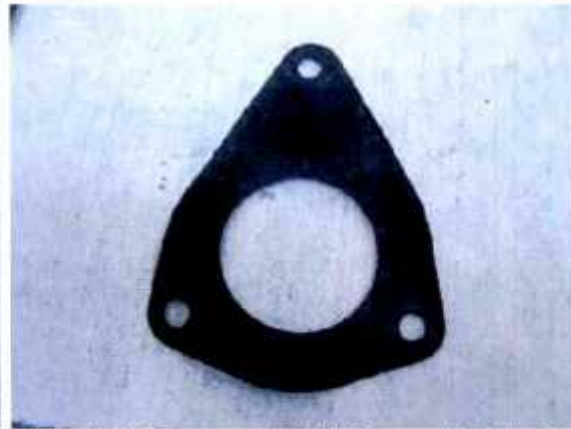
Figure AI-16: Pump / control interface gasket (side 1)
