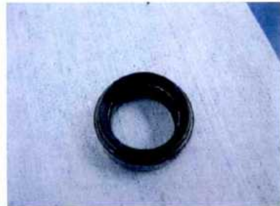
Figure AI-24: Main drive shaft seal
