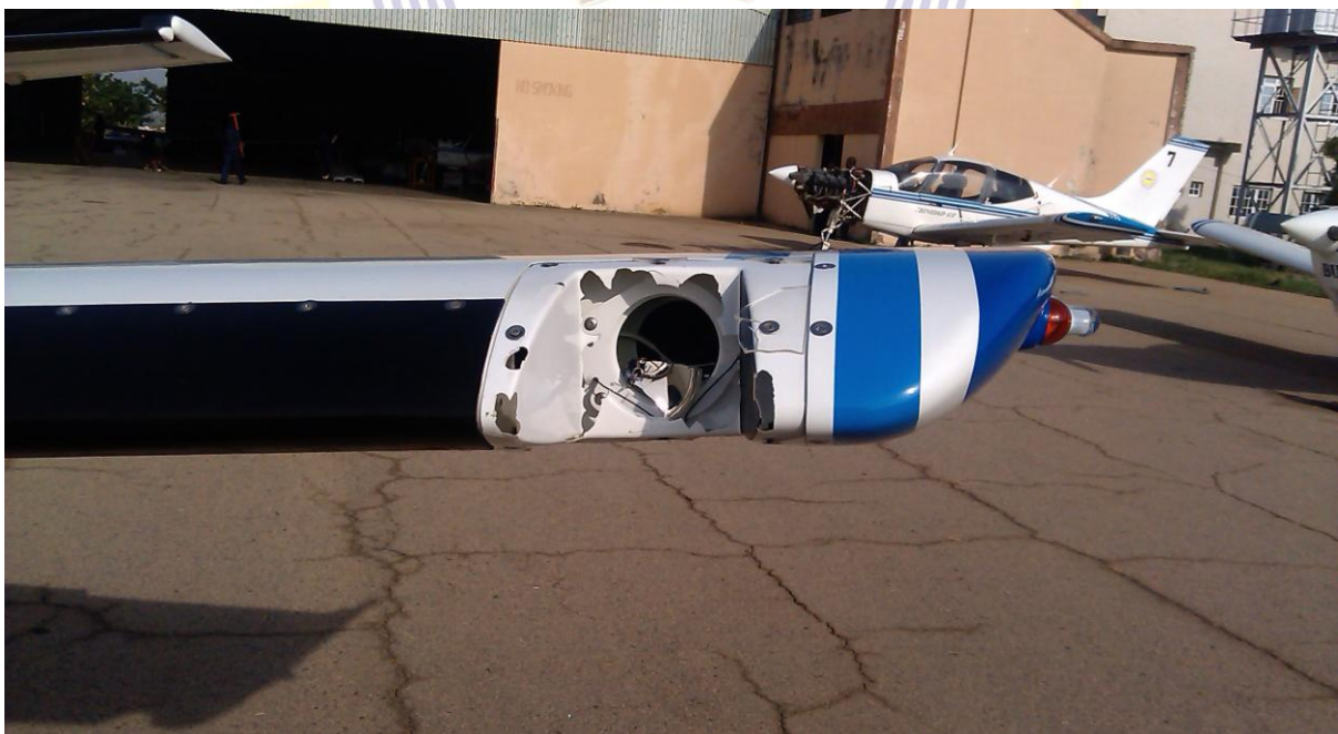
Figure 4: Picture showing damaged Left Landing Lamp housing
