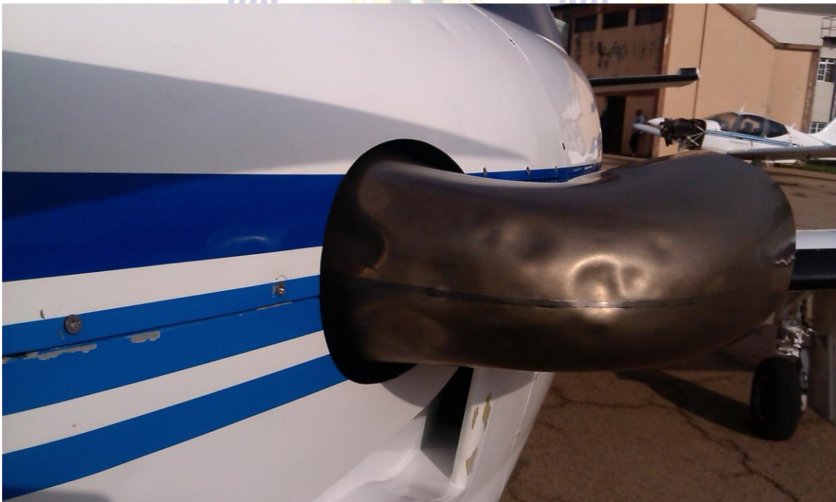
Figure 2: Picture showing dented Right Exhaust stack
