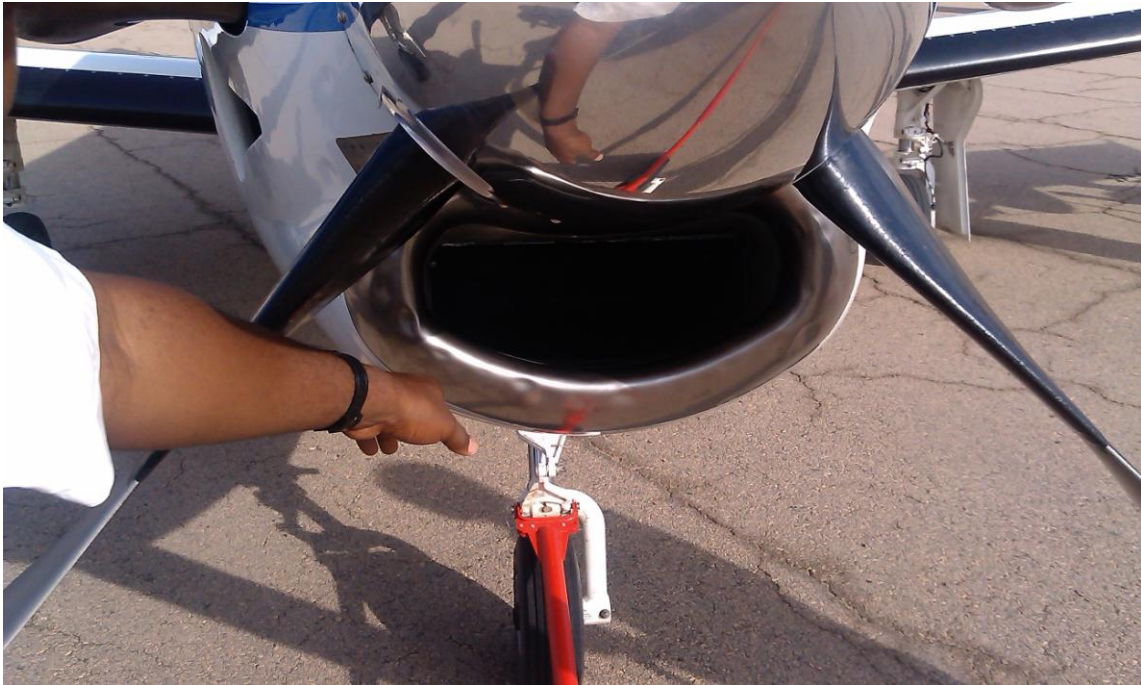
Figure 5: Picture showing dented Lower Engine Cowl assembly
