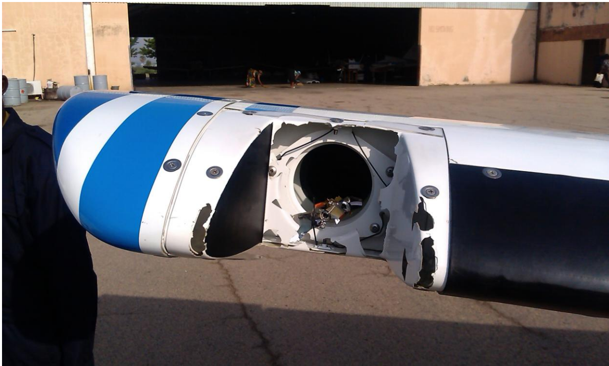
Figure 3: Picture showing damaged Right Landing Lamp housing
