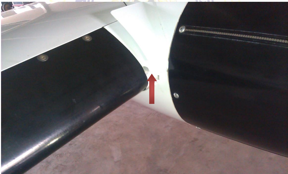
Figure 6: Picture showing dented Right Wing root Leading Edge section (red arrow)
