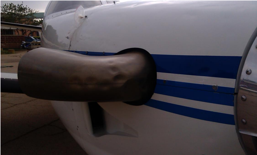
Figure 1: Picture showing dented Left Exhaust stack
