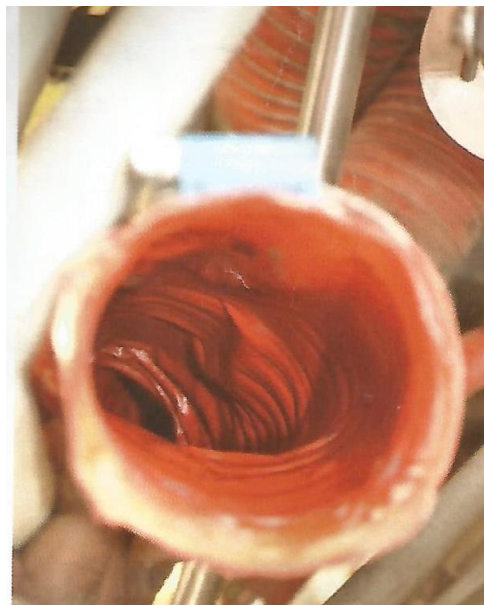
Figure 3: Delaminated turbocharger hose found installed on 5N-BRD
