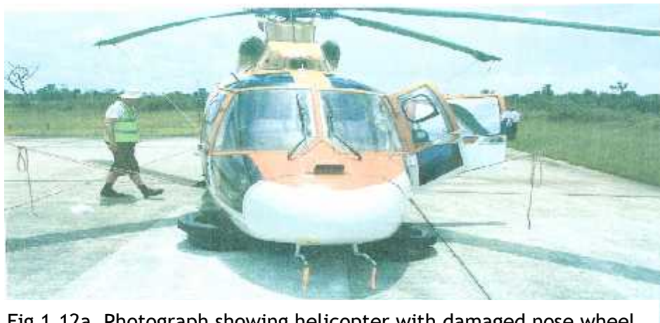
Fig 1.12a Photograph showing helicopter with damaged nose wheel
