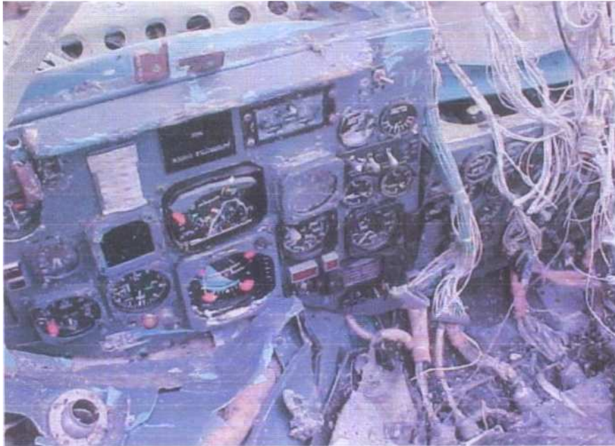
Photograph showing the Instrument panel found on taxiway, 330m away from the rest of the wreckage
