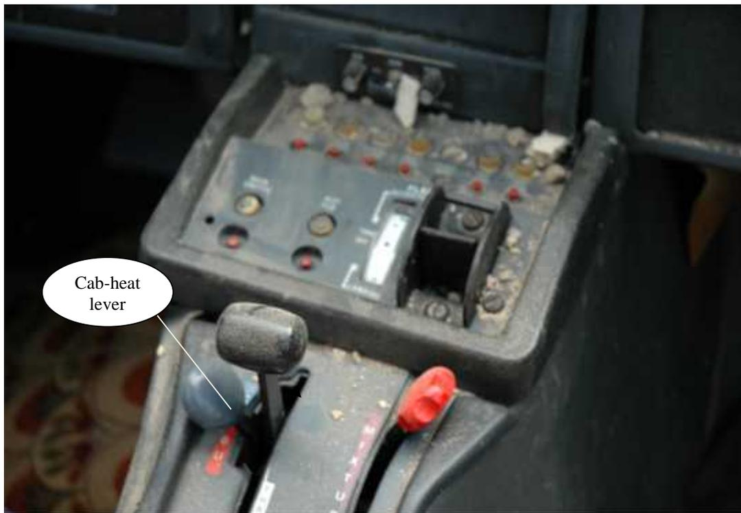
Photograph showing cab-heat lever in mid position
