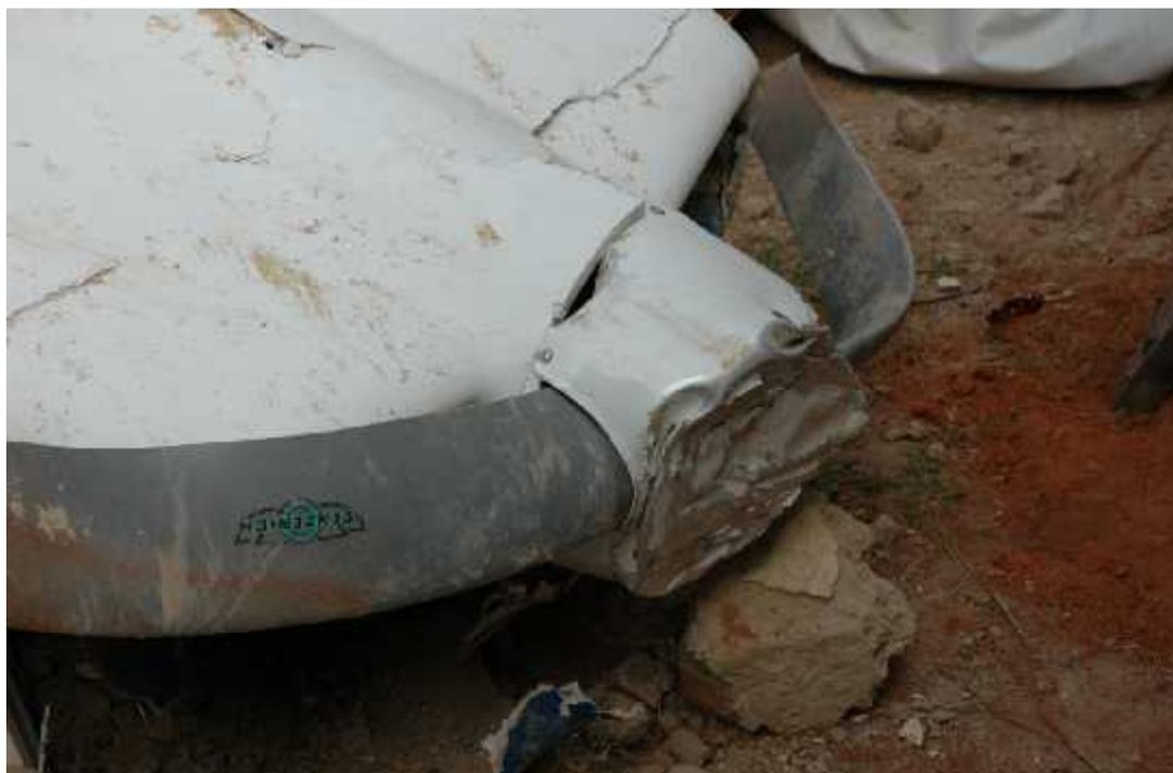
Photograph showing damaged propeller blades
