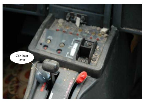
Photograph showing cab-heat lever in mid position
