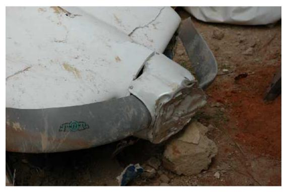
Photograph showing damaged propeller blades
