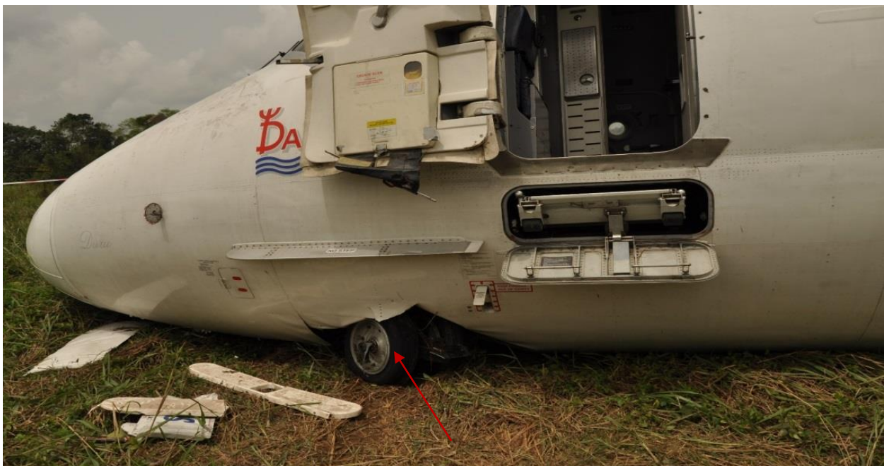
Figure 2: Collapsed nose wheel of the aircraft
