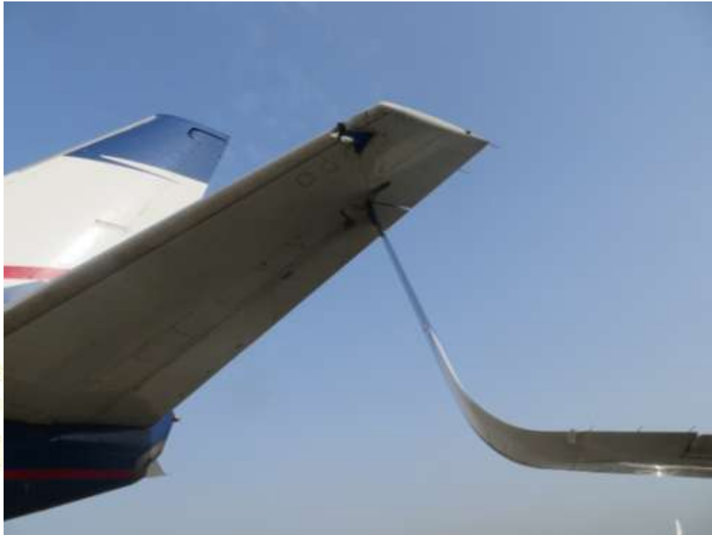
Figure 1: Picture showing damage to the leading edge of horizontal stabilizer of 5N-BQP and the winglet tip of 5N-BQR
