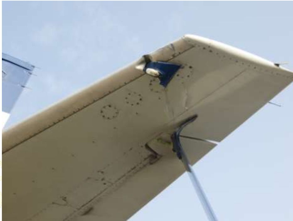
Figure 2: Picture showing damage to the leading edge and skin of horizontal stabilizer of 5N-BQP
