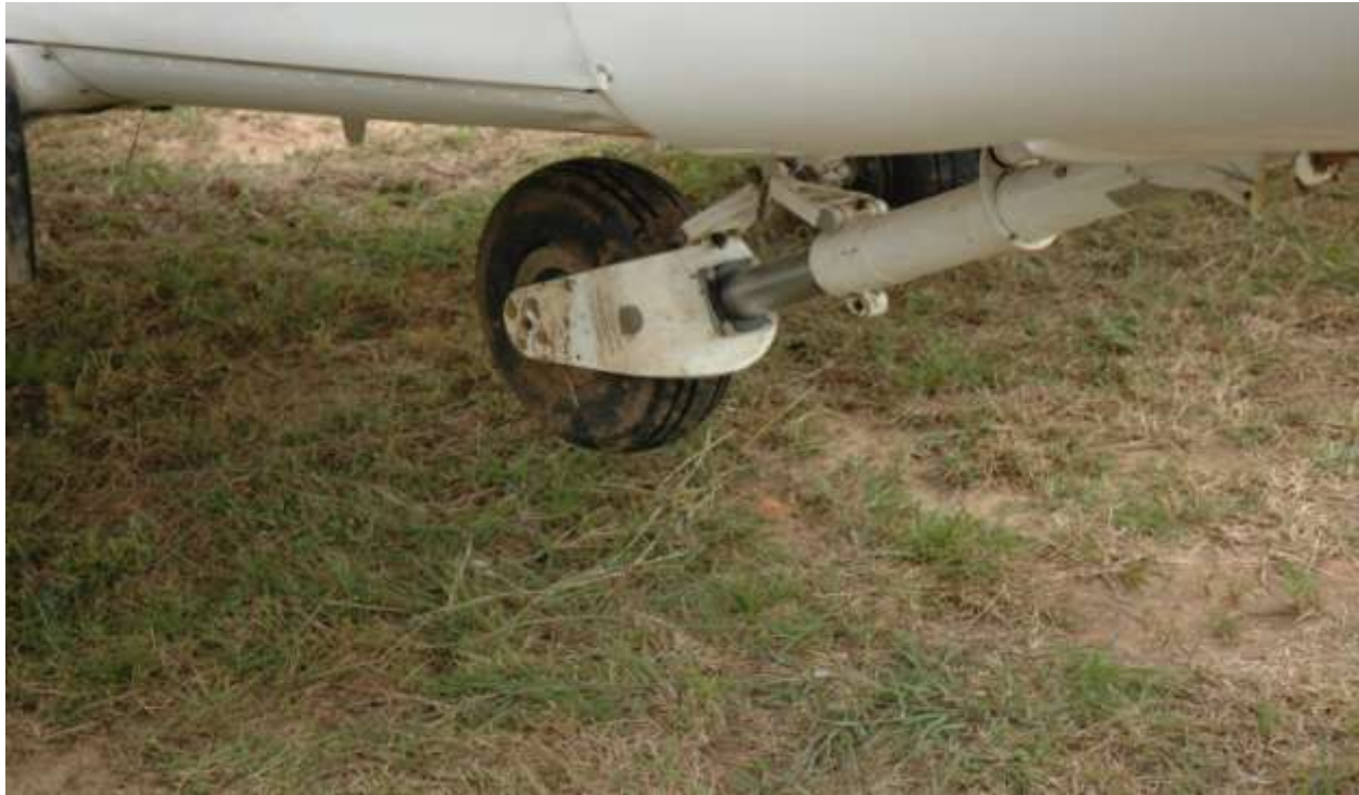
Figure 4: Picture showing damaged nose wheel landing gear
