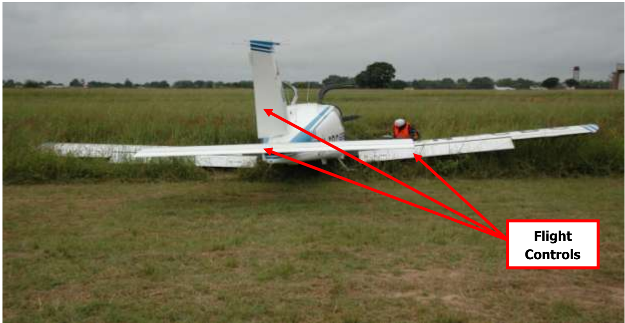
Figure 2: Rear view of the aircraft showing the position of the flight controls
