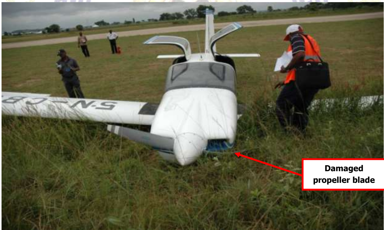
Figure 3: Nose dome area of the aircraft showing damage to propeller blade
